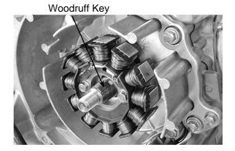
Install the flywheel onto the crankshaft with the flywheel hole aligned with the crankshaft woodruff key.
