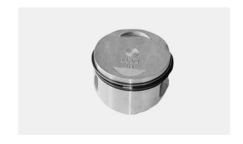
Install the piston rings onto the piston and measure the piston ring-to-groove clearance.
