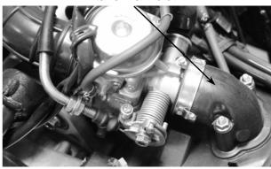
Remove the cooling fan cover. (⇒14-7) Remove the engine cover bolts and screws. Separate the engine cover joint claws.
