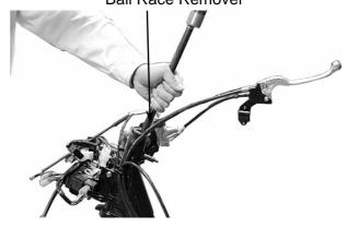
Drive new top and bottom ball races into the steering head using the outer driver.
