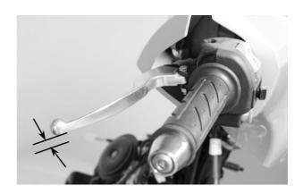
If the free play do not fall within the limit, adjust by turning the adjusting nut.
