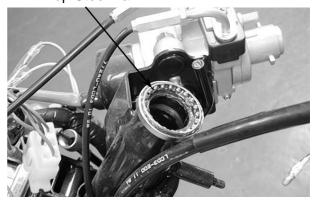
Apply grease to the ball races and install the front fork.
