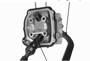
Valve Spring Compressor Attachment
