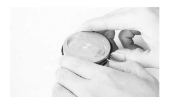
Remove the piston rings and insert each piston ring into the cylinder bottom.
