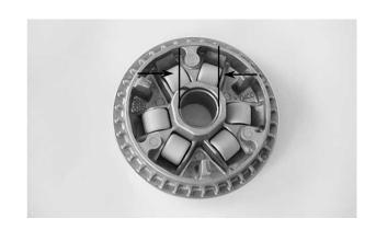
Check the drive pulley bushing for wear or damage.
