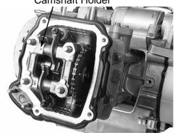
Remove the camshaft gear from the cam chain and remove the camshaft.
