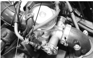
Air Cleaner Connecting Intake Manifold Band Tube Band
