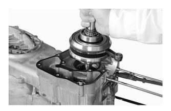
Clean off all gasket material from the crankcase mating surfaces.
