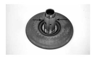
Check the movable driven face for wear or damage.
