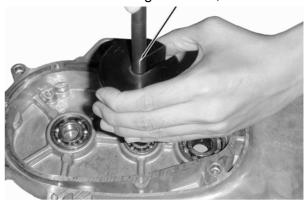
Drive new bearings into the left crankcase. Install a new drive shaft oil seal.
