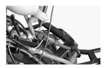
Measure the secondary coil resistances with and without the spark plug cap.
