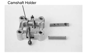
Measure the I.D. of each valve rocker arm.
