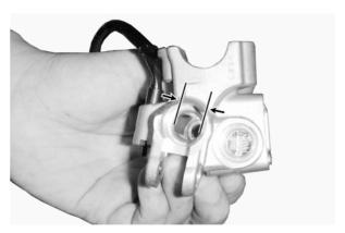
Measure the brake master cylinder piston O.D.
